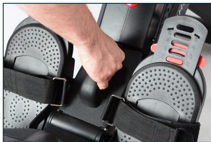
17. To lock into place, pull up on this handle until you hear a click. Once you hear the click, the rower is safe to use.
